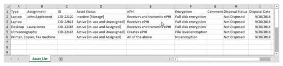
It is important to remember that files must be kept in CSV format to work with the SRA Tool. **The tool does** not accept .XLS or .XLSX files. Ensure that files retain the .CSV extension and file type.
